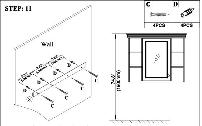
Draw the spacing between the walls and the No.8, punch holes in the wall, and fix the No.8 to the wall with screws.
