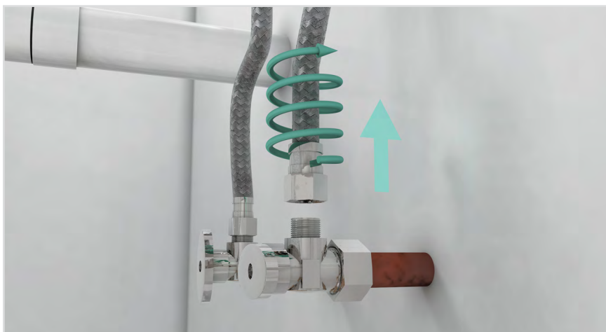
Diagram 2.3(B).5 Detach Cold Water Feed Line
