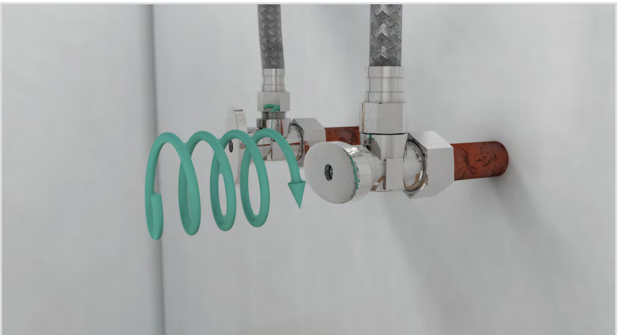
Diagram 2.3(B).4 Shutoff Cold Water Source Valve
