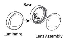
Rotate the lens assembly counter clockwise until it is stops and then lift the lens assembly straight off.
