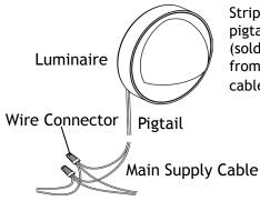
Strip both leads from the luminaire pigtail. Using two wire connectors (sold separately), connect the leads from the luminaire to the main supply cable leads.
