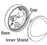
Push the lens assembly back onto the base aligned with the gaps on the base. Push hard (moisture proof fixture requires force to get air out). Once the lens assembly is flush with the base, rotate the lens assembly until it stops and locks into place.
