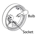
Insert the bulb with correct wattage and type marked on the luminaire label.
