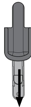
Slide the cradle onto the mounted bracket.
