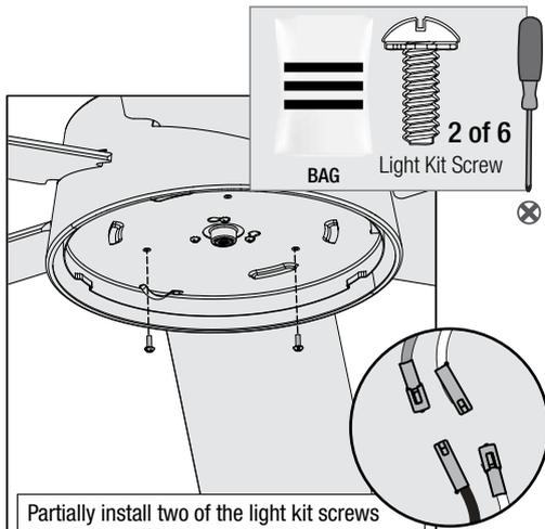
Partially install two of the light kit screws found in the hardware bag. It does not matter which two screw holes you choose. Connect the single-pin connectors from the LED assembly to the connectors from the fan. Connect the white wires together. Connect the blue and black wires together.
