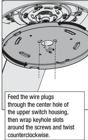
Feed the wire plugs through the center hole of the upper switch housing, then wrap keyhole slots around the screws and twist counterclockwise.
