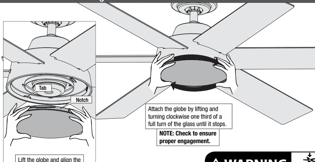
Lift the globe and align the notches in the globe with the tabs in the light kit.
