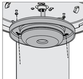
Align the keyhole slots in the light kit housing with the two screws. Make sure all the wires from the fan and the light kit are snug inside the center of the light kit, not pinched in between the upper switch housing and the light kit or hanging out of the sides.
