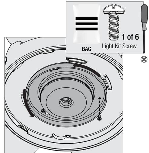
Turn the light kit counterclockwise until the light kit screws are firmly situated in the narrow end of the keyhole slots. Install the third screw and tighten all three screws securely.
