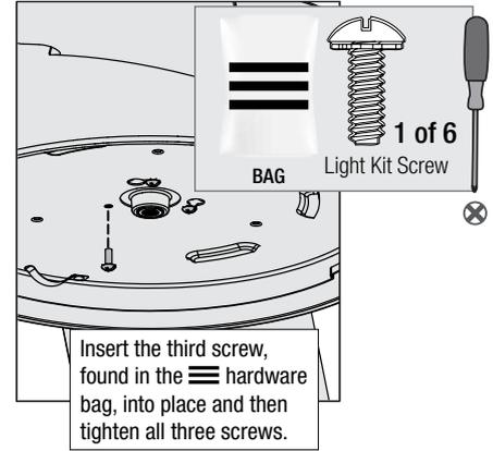
Insert the third screw, found in the hardware bag, into place and then tighten all three screws.
