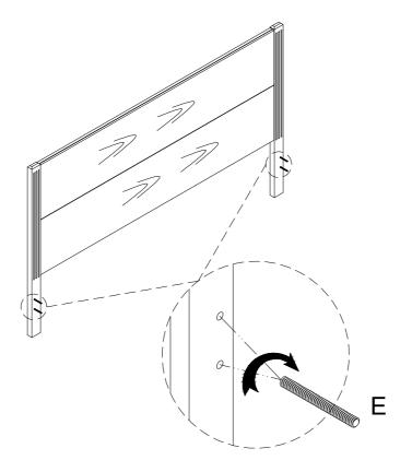
As shown in the figure, place F and G inside the hole, insert E and then connect it with F and G. Please make sure they do not loose or fall out when twisted.
