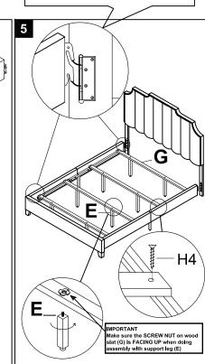
For correct assembly please ensure the double hooks are latched properly.
