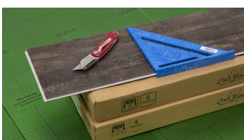
Cutting boards using Score and Snap technique
