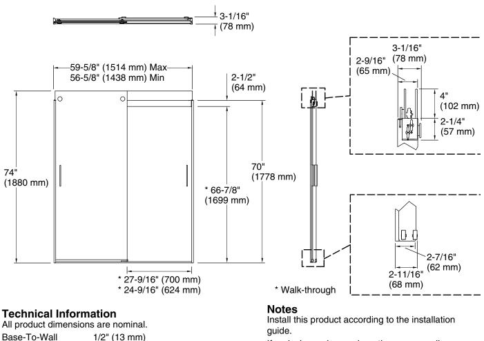
If replacing a shower door, the narrow wall jamb design of this door may not cover the existing shower door holes.
