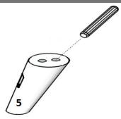
Insert (1) Wood Dowel (Part D) into the upper hole in Front and Back Legs (Part 5)
