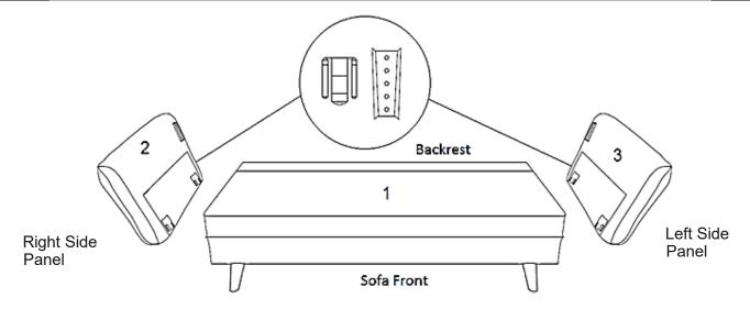
Return sofa to the upright position and insert the brackets on the Right Side Panel (Part 2) and Left Side Panel (Part 3) into the Receiver Brackets on the side of the Sofa.
