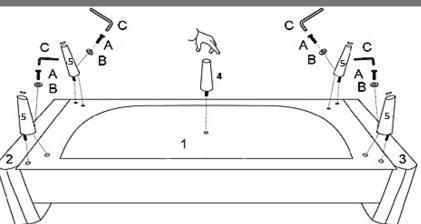
Insert Center Leg (Part 4) into the Middle of the underside of the Sofa Seat and turn clockwise to tighten.
