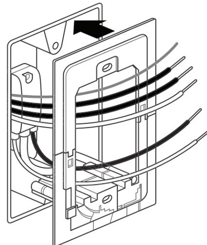
**NOTE:** Surround is in two pieces to aid in assembly when **adorne**<sup>™</sup> devices have been previously installed.
