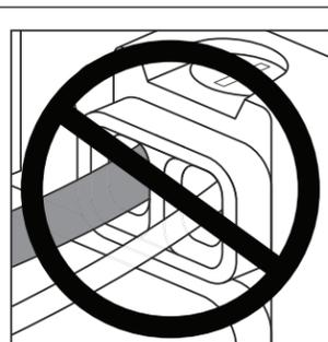
**WARNING:** Do not pair different size wires in the same terminal. If stranded wire is used, always pair the Accent Light wire with the stranded wire.
