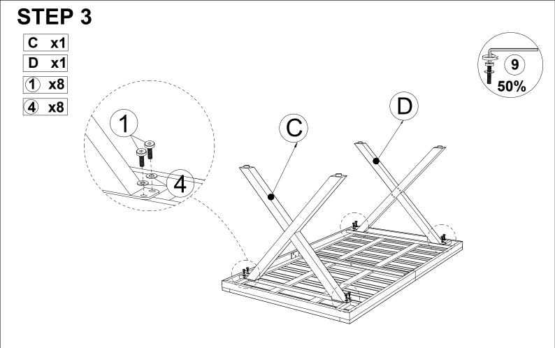
Connect the Part from Step 2 & the Leg Table (C),(D) tighten Bolt (1) & flat Washer (4) & Allen Key (9).
