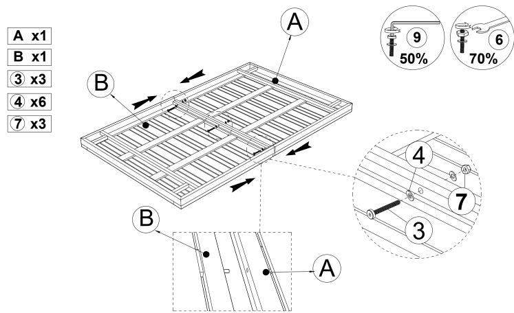
Connect Top Right Table (A) & Top Left Table (B), tighten Bolt (3) & flat washer (4),Nut (7),Key (6) with Allen Key (9).
