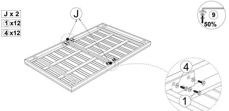
Connect the Part from Step 1 & Flat Connector (J), tighten Bolt (1) & flat washer (4) with Allen Key (9).
