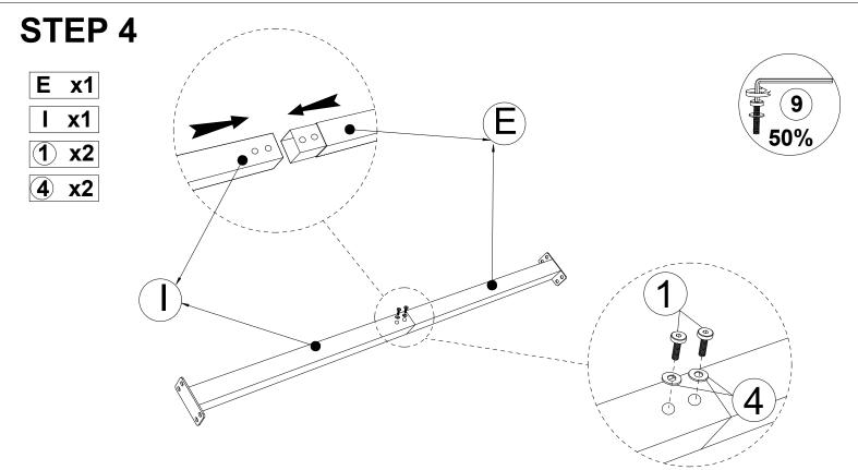
Connect the Half Bar 1 (E) & the Half Bar 2 (I), tighten Bolt (1) & flat Washer (4) & Allen Key (9).
