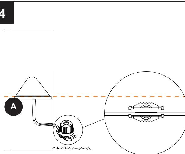
Insert wire from low-voltage transformer (sold separately) into the wire guide by twisting the wire into each end of the wire guide. Align the pins on the connector top cover so that each pin lines up with opposite sides of the wire. Securely tighten the connector top cover making sure the pins completely pierce the plastic shield of the wire.
