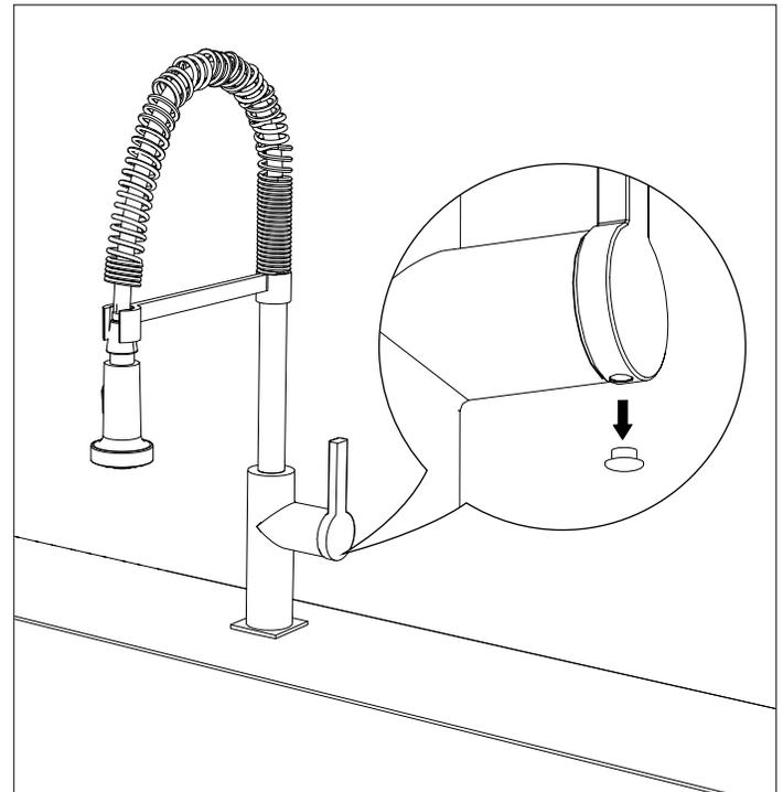
**2** Loosen the inset handle screw and remove the handle.
