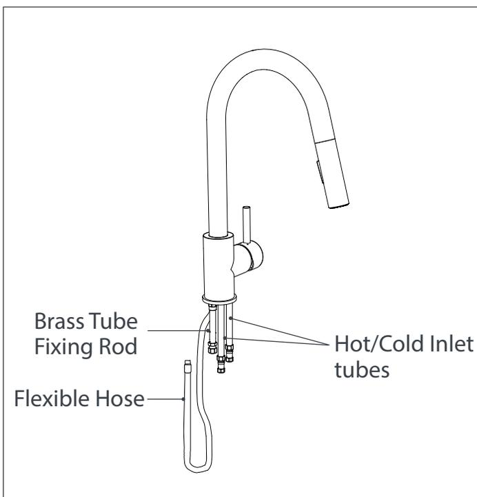
**3** Add the Faucet Collar and O-ring to the Faucet assembly and connect hot/cold Braided hoses to the inlet tubes.
