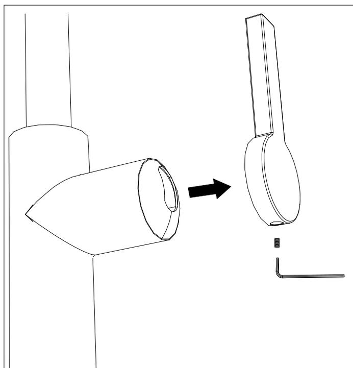
**3** Unscrew and remove the cartridge cover and O-ring.
