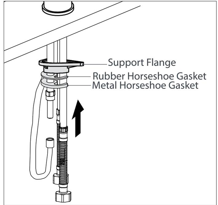
**7** Connect the flexible hose to the Brass Tube fixing rod.
