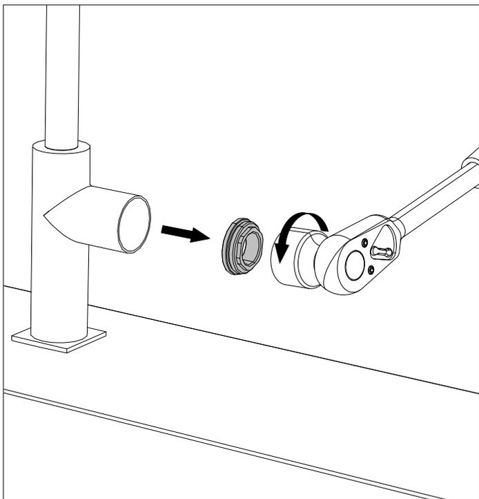
**5** Remove the cartridge from the handle.
