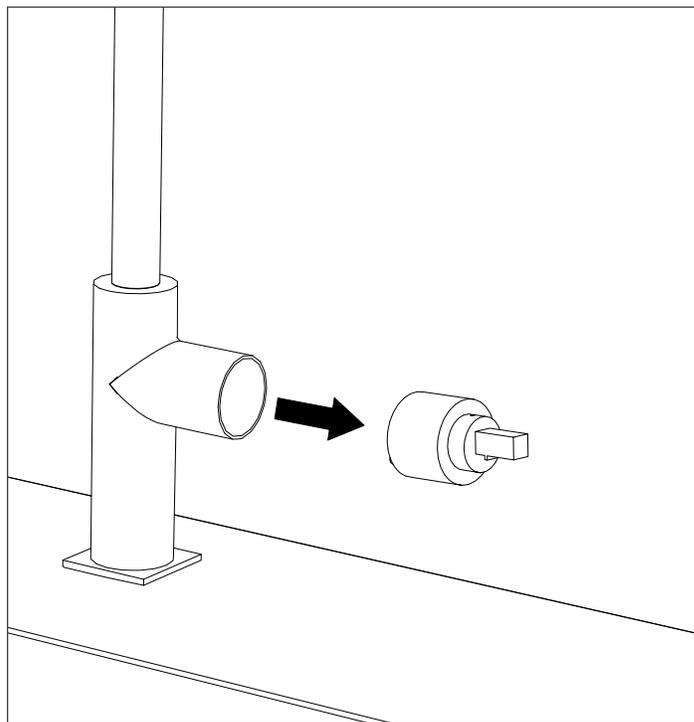
**6** Replace the cartridge and reassemble the handle assembly as shown below.
