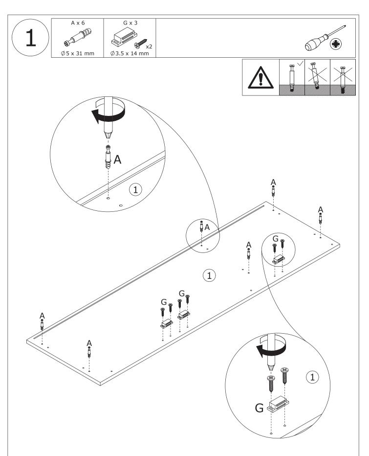
Screw eccentric rod(A) board 1 with a screwdriver as shown. Fix part(G) to board 1 as shown.
