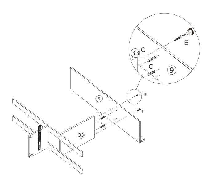
Knock wooden dowel(C) into plate 9 at first, then attach to plate 33 and fix with screw(E) as shown.
