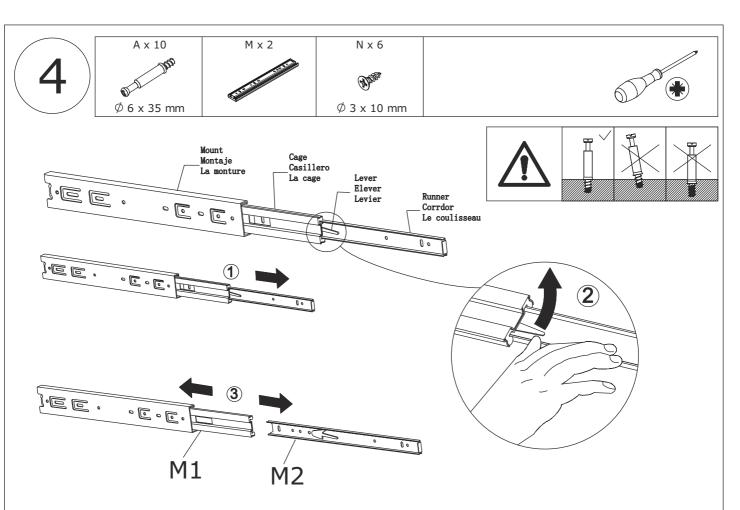
Fix slide rail(M1) to plate 3 and 4 with screw(N) as shown.
