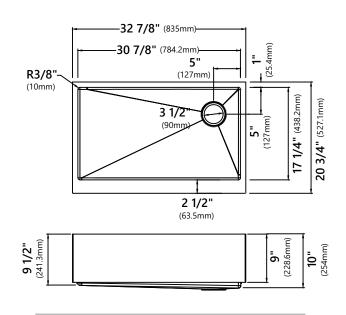
Model #: KHF410-33 Sink Dimensions: 32 7/8" x 20 3/4" x 10" Min Cabinet Size: 36"
