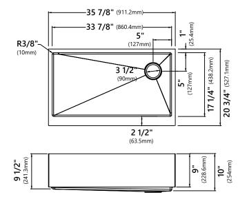
Model #: KHF410-36\* Sink Dimensions: 35 7/8" x 20 3/4" x 10" Min Cabinet Size: 39"
