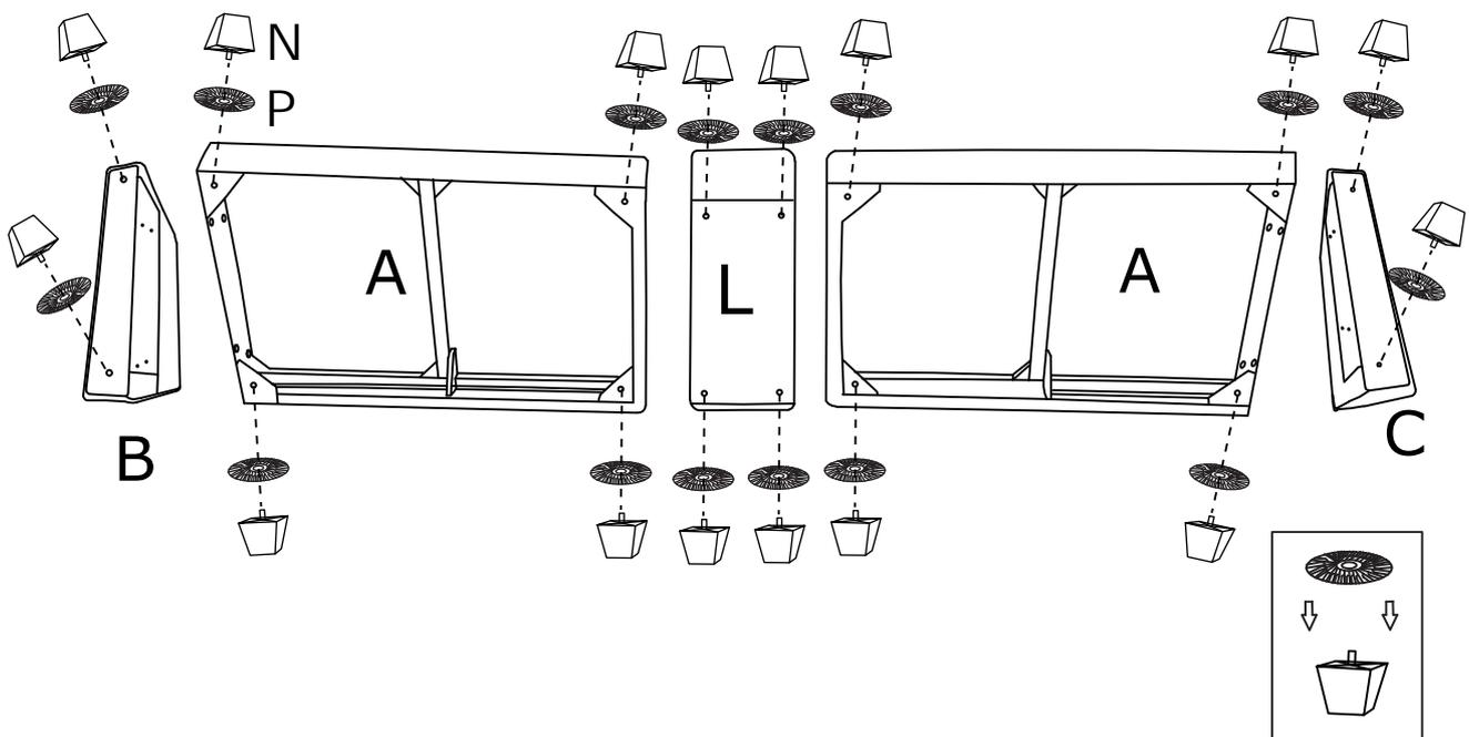
STEP 3: Assemble the Legs (N) on the Ottoman frame (H) with Gaskets (P) .
