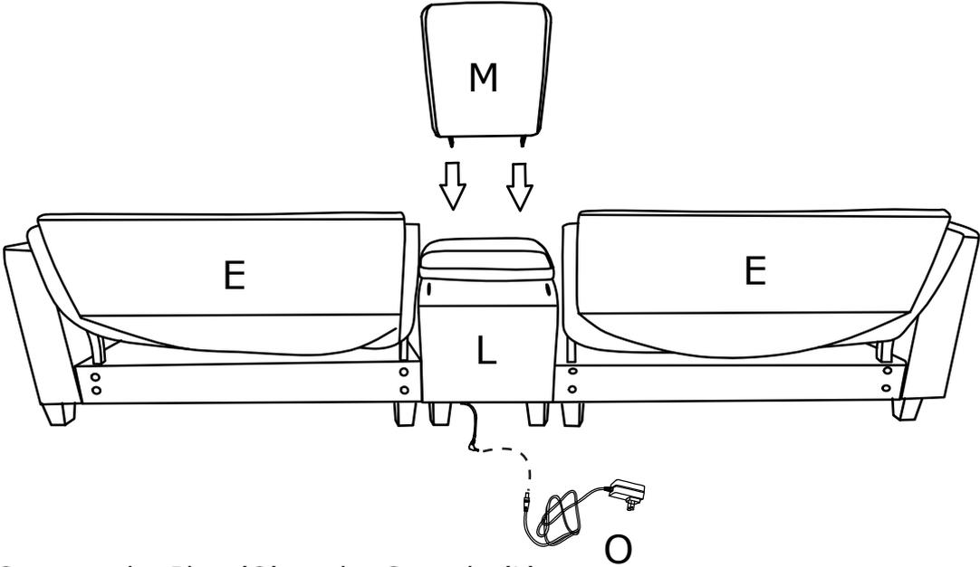
Connect the Plug (O) to the Console (L).
