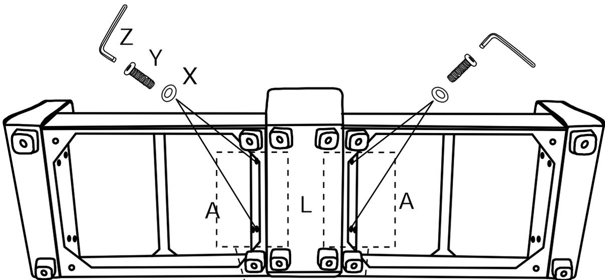
Align the seat frame holes when attaching the seat frame to the console.
