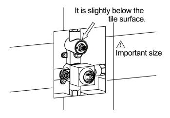
4. The water outlet of the hand shower is slightly lower than the tile surface.
