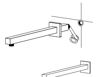
Before installing the product, please be sure to remove sundries and sludge from the water pipe to prevent sundries from blocking the product.
