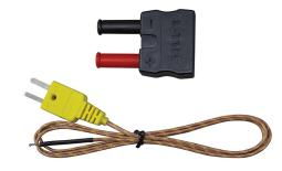
Specific for HVAC applications, this High Temperature Thermocouple (and other Klein K-Type Accessories) extend working temperature ranges for Klein's HVAC Digital Multimeters and Clamp Meters. These accessories work with all Klein digital multimeters and clamp meters that measure temperature, as well as any other brand with meters that measure temperature. Other accessories include Temperature Pipe Clamp, Temperature Probe and Banana Plug Adapter.
