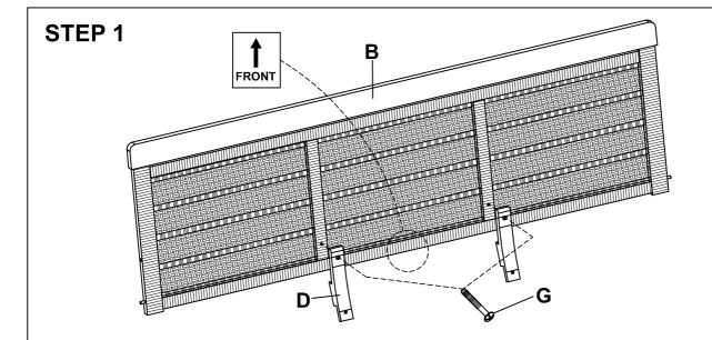
Attach back support (B) and back support holder (D), secure using 1 1/4" bolt (G), as shown. Tighten all bolts using screwdriver.
