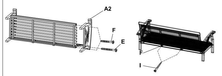
Attach left side frame (A2) into pre-assembled frame, secure using 3 1/2" bolts (E) and 2" Bolts (F), Attach back support holder (D) and seat (C) secure using 1" screw (I) as shown. Tighten all bolts and screws using screwdriver.
