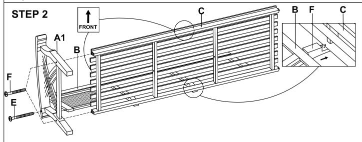
Attach back support (B) and seat (C) into right side frame (A1), secure using 3 1/2" bolts (E) and 2" Bolts (F), as shown. Tighten all bolts using screwdriver.
