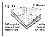
between the closure strips. Turn sheets or tiles right side up, carefully lay in place so caulked closures seat on flashing, and nail in place.
