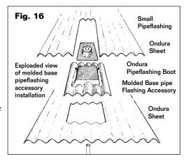
directly over the sheet to which the accessory is applied, be caulked to the accessory, and its upper end should be under the lap of the next higher row of Ondura sheets. Fasten with Ondura nails (see Fig. 16).
