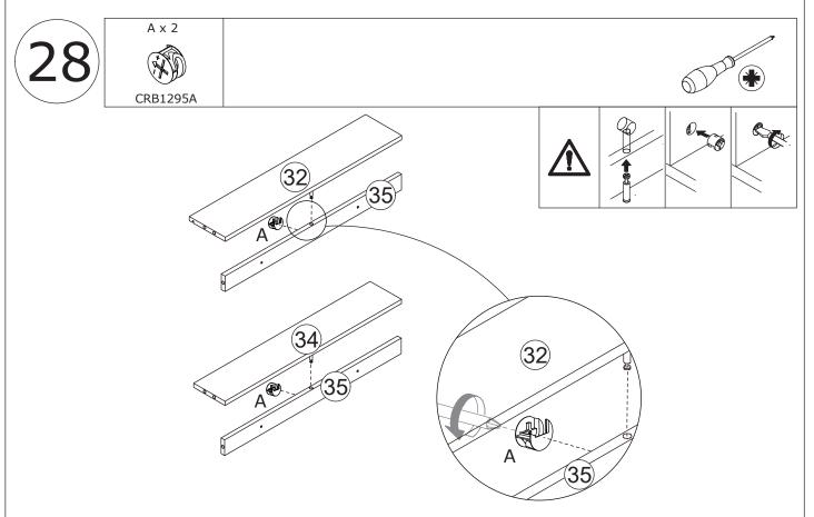
Attach board 32 and board 34 to board 35 respectively and turn cam locks(A) clockwise to tighten as shown.
