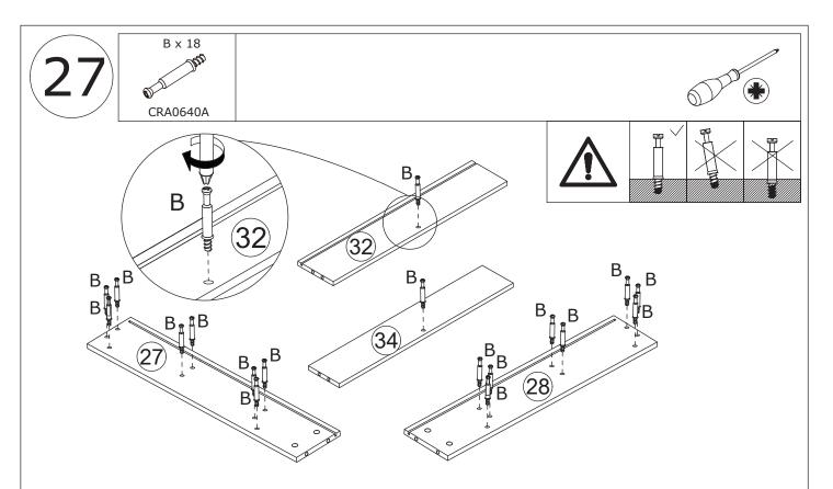
Insert quickfit screw(B) into corresponding holes in board 27,28,32,34 with a screwdriver as shown.
