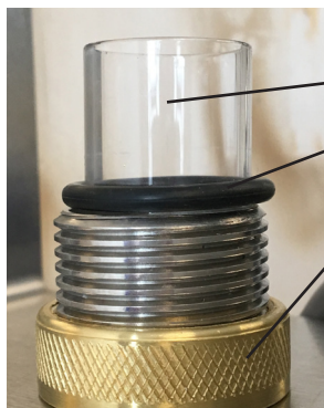
2) Quartz Sleeve inserted into UV Chamber Quartz Sleeve Black O-Ring Locking Nut
