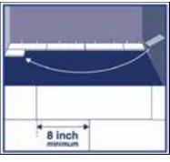
**Step 3:** Use leftover plank from first row as starter for second row. Minimum 8" stagger between plank end joints.
