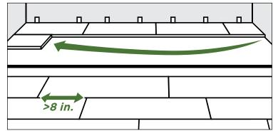
Tap the length end to ensure a tight fit, then tap the short end to drive down the short end tongue into groove.
