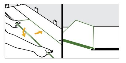
Start your second row. With a cut-off that is more than 8" long or start with a new plank.
