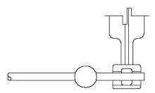
Install the complete pop-up assembly without the stopper. Drop the stopper in the pop-up so that the bottom ledge of the stopper rests on top of the pivot rod.
