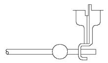
Before installing the pivot rod and strap assembly, insert the stopper into the pop-up. Assemble pivot strap assembly to pop-up body so that the rod goes through the lower opening of the stopper.
