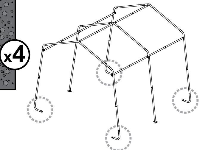
**NOTE:** For best results ShelterLogic recommends additional anchors, one for each foot plate, for a stronger, more secure installation.
