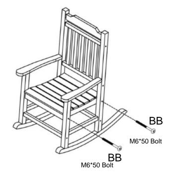
Attach the Backrest (Part F) to the Leg (Part A) using (2) M6\*50 Bolts (Part BB). Attach the Crossbeam (Part C) and (Part D) to the Leg (Part B) using (2) M6\*50 Bolts (Part BB).
