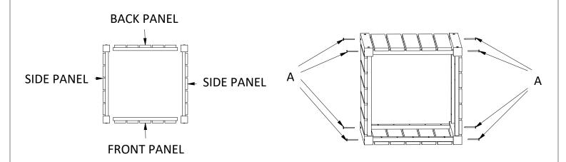
**1.)** Place the Front Panel on the ground with the inside facing up. Insert 2 (A) Bolts on each side through the Side Panel and tighten. Repeat for the Back Panel
