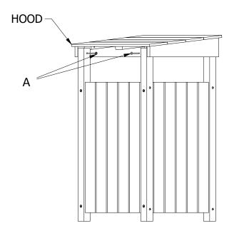
**5.)** For Trash Cans with the Hood, Place the Hood on top as shown and attach 2 (A) bolts
