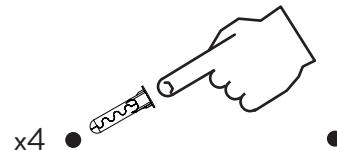
**4** Insert the screws into the bottom two drilled holes and secure with a screwdriver. Hang the mailbox onto the secured screws using the bottom eyelet holes on the back of the mailbox.
