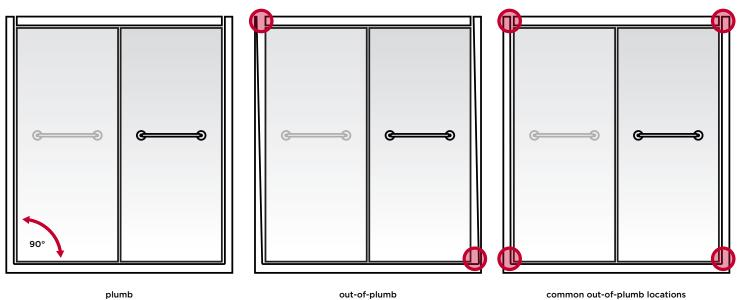
Most Delta Shower Doors are designed to accommodate out-of-plumb conditions up to 3/8". If needed for proper alignment, each roller can be individually adjusted from inside the shower enclosure. Always follow the safety guidelines, and for more detailed instructions, refer to installation guide or contact our Delta Shower Doors Customer Care with guestions 800-964-4850.
