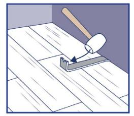
Step 9: Use hammer and pull bar to lock long edges of flooring on final row.
