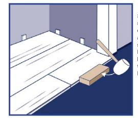
Step 1: Undercut space under door jamb to allow flooring to slide freely. Tap long edge with hammer and tapping block to lock long edge.
