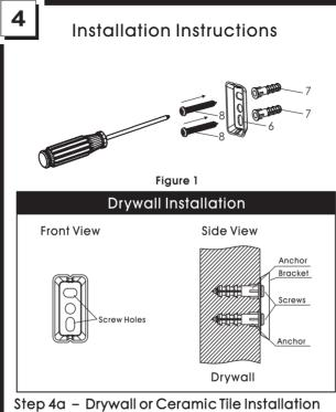
the marked spots drill 1/4" holes in the wall, then insert the insert anchors(7) in the holes, u the hammer to tap them into place. (Be sure not to hit them too hard)
