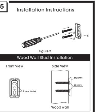
Step 4b – Wood Wall Stud Installation Drill 1/16" holes in the marked spots, be sure to keep the drill level. Insert anchors will not be needed.
