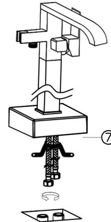
7. Drill holes and use the explosion screw to fix the base on the ground then put the decorative cover over the base
