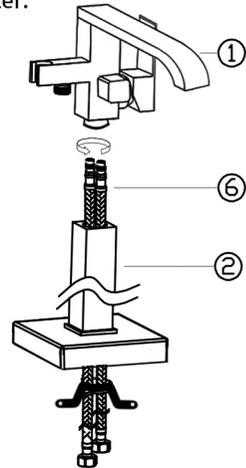
3. Prepare water supply pipes like the drawing below. (unit:mm)
