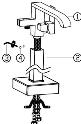
5. Screw the base to the straight pipe.
