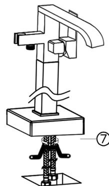
6. Connect another side of the water supply hoses to the water supply pipe. Make sure they were screwed into the correct outlets for hot water and cold water
