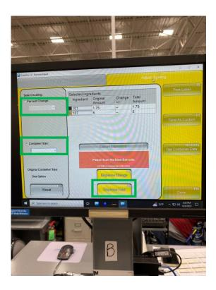
Step 4: From the drop-down menus on the left, select **Percent Change or Container Size** to change amount of colorant dispensed based on percent or the size of the container. Once the selection has been made select **Dispense Total.**
