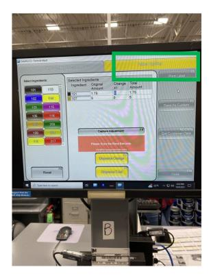
Step 3: From this screen, select **Adjust Scaling** to change amount of colorant dispensed.
