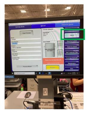
Step 2: Select **Adjust** from the main screen to input changes for colorant percentage or container size.
