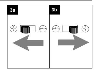
3c. **IMPORTANT**: Reverse switch must be set either *completely LEFT* or *completely RIGHT* for fan to function. If the reverse switch is set in the *middle* position, fan will not operate.
