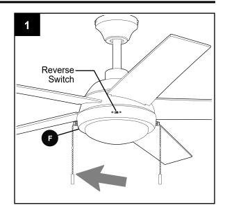
2. The pull chain located to the right of the reverse switch on the switch housing (F) is labeled LIGHT and is used to control the light.
