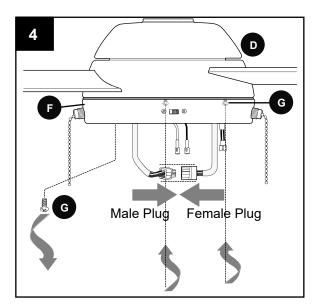
Locate BLUE and WHITE wires in switch housing (F). Connect WHITE wire from LED light kit (I) to WHITE wire from switch housing (F). Connect BLUE wire from LED light kit (I) to BLUE wire from switch housing (F). Make sure molex connections are secure.
