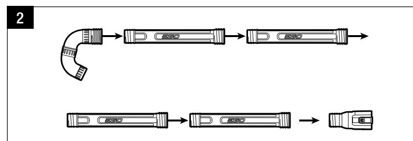
2. Align the groove in the gutter cleaning attachment kit and push the tube onto the blower housing until you hear a "click" (Fig.3&4).
