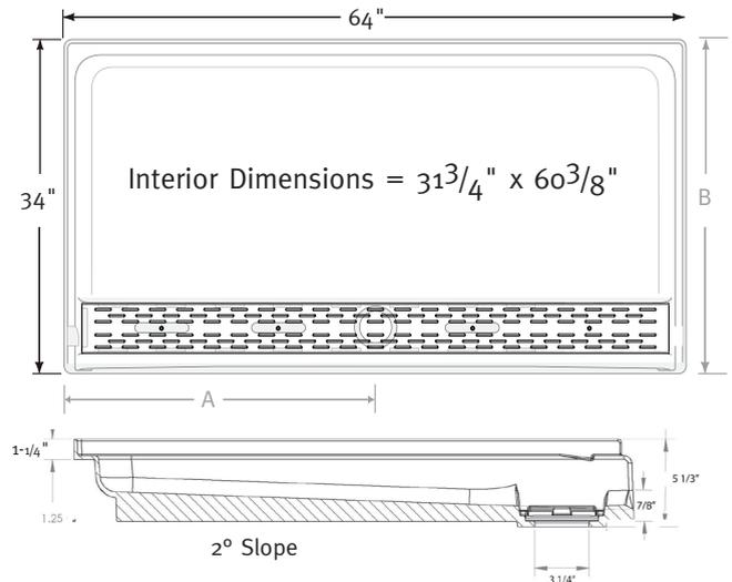
Trough system drains into standard 2" drain pipe.
