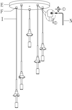
5 » If needed, shorten the extra length of the fixture wires from cord (I) so that they all are at least 6 inches (152.4 mm) long above canopy (E) within the outlet box.
