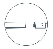
Unplug the power supply and remove the plastic end cap cover. Attach extension to the Light Strip.
