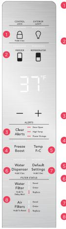
Use to lock the display. Press and hold a for 3 seconds to enable/disable. The indicator flashes and an alert sounds when **CONTROL LOCK** is enabled. You can't make changes on the display while the lock is engaged. Select compartment for temperature
