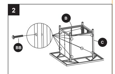
Once all bolts have been installed and hand tightened, go back and tighten firmly with wrench, EE.
