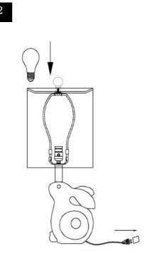
Step 2 Insert the bulb(G) into the socket(C).
