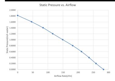
\* Max velocity CFM of blower measure in open air environment\*
