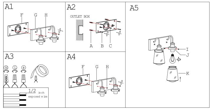
Step A1 » Unscrew knob nuts (H) from back plate (G) then gently remove mounting plate (F). Then set them aside for later installation.
