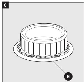
7. Insert the pop-up body (H) into the sink and screw the flange (E) onto the pop-up body (H). Ensure the pivot hole is facing the back of the sink. Tighten the nut (G) and remove the pivot nut (I).
