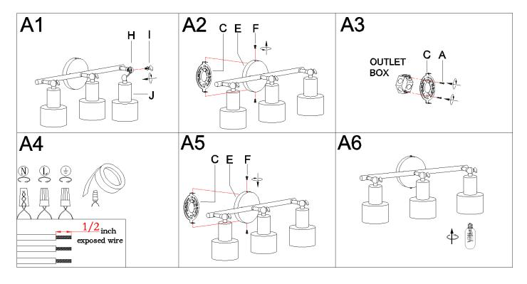
Step A1: Adjust the fixture wires in joints (H).
