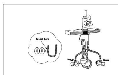
5. Take the weight out and press down "open" side then clasp weight to the label place "WeightHere" lnstallation finish and test leak or not.
