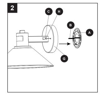
Use the bracket screws (RR) to attach the mounting bracket (A) securely to the outlet box (sold separately). Note: In order for fixture (D) to be level, the mounting screws (B) must be aligned exactly perpendicular to the horizon since they will determine the orientation of the fixture.
