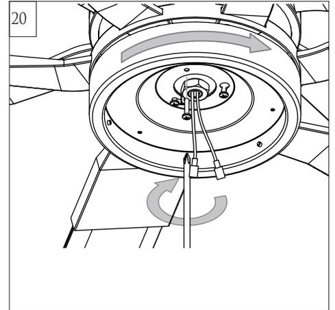
Install the light pan. Align its key holes with the set screws on the plate and reinstall the screw removed in step 18. Tighten screws securely.
