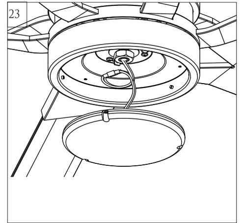
**Caution:** Corresponding to next installation step, tuck the lead wires into the light pan as shown in illustration and make sure the light lead wires are not pinched between the light pan and the LED light fixture.
