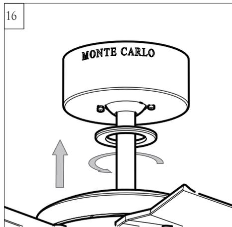
Lift canopy up, aligning its keyhole slot with the preassembled screw on mounting bracket and twist counterclockwise to lock in place. Reinstall the screw removed in step 15 and tighten all screws securely. Attach canopy bottom cap onto canopy by aligning its notch with the screws on mounting bracket and twist clockwise till tight.
