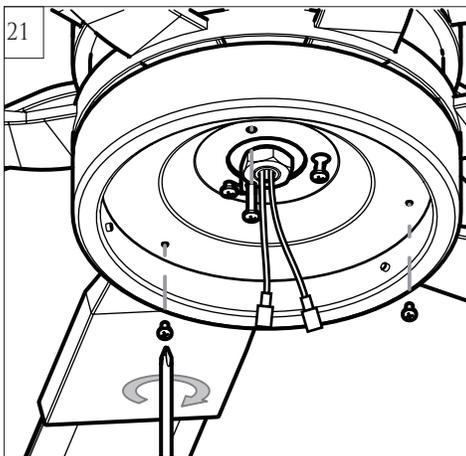
Removed set screws from light pan. Keep screws.
