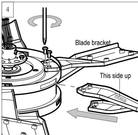
Place motor assembly on a suitable area of Styrofoam and Install blade brackets. Insert blade bracket into the slots on flywheel, aligning the holes on blade bracket with the screw holes on flywheel (**both top and bottom sides**), and then partially install set screws provided. Tighten set screws securely once the blade bracket is installed in position with the set screws.
