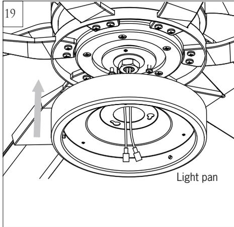
Place light pan over lead wires
