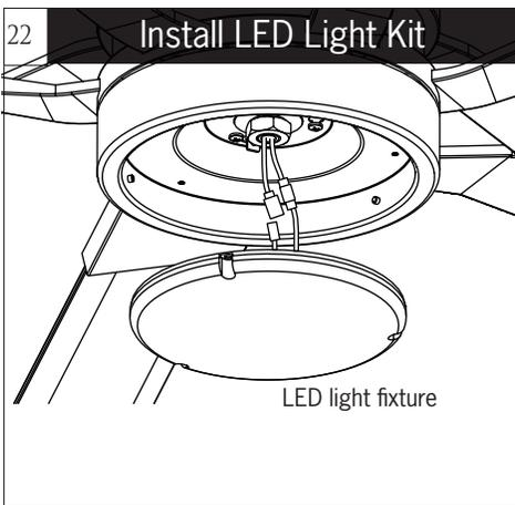
Connect white wire from fan to white wire from LED light fixture and then connect blue (or black) wire from fan to blue (or black) wire from LED light fixture.
