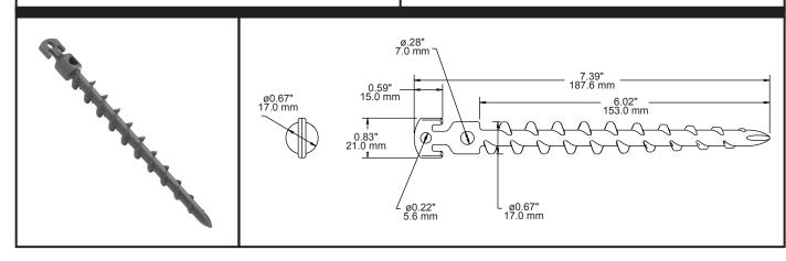
MATERIALS: Tent Anchor is fabricated from injection molded 20% glass filled nylon material.
